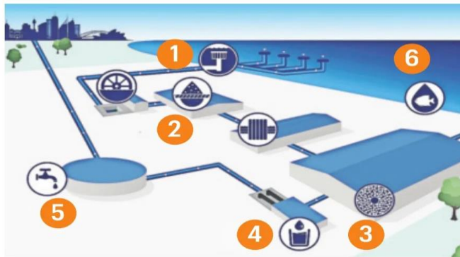
1. Seawater intake 2. Pre-treatment filtration to remove particulate matter 3. Reverse osmosis to remove salt, minerals 4. Post-treatment for consumption readiness 5. Drinking water delivery 6. Seawater concentrate outlet (SYDNEY DESALINATION PLANT AS REFERENCE)
